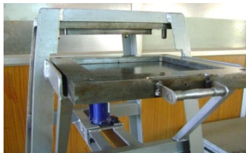
Fig 2. Die used for preparing specimens
